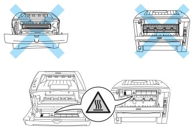
There are high voltage electrodes inside the printer. Before you clean the printer, clear a paper jam or replace parts, make sure you have turned off the power switch and unplugged the printer from the AC power outlet.
